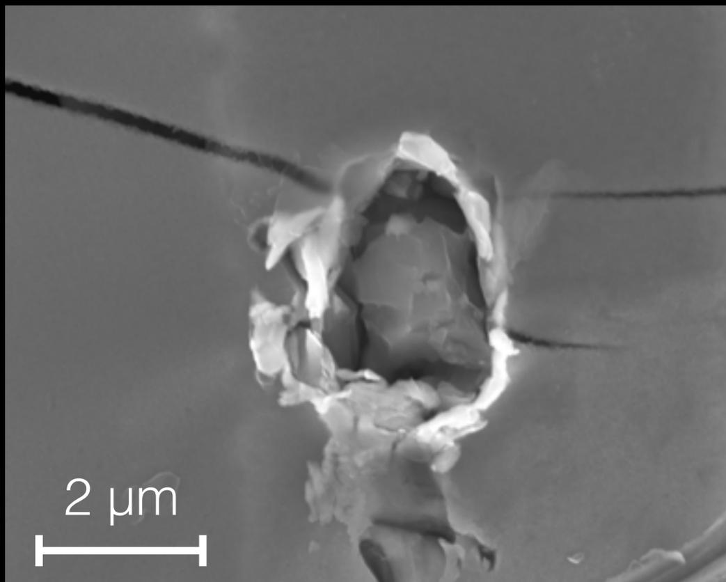
Meteoritic ejecta captured into Cu wire on TEM grid. Image width = 10  $\mu\text{m}$ .
