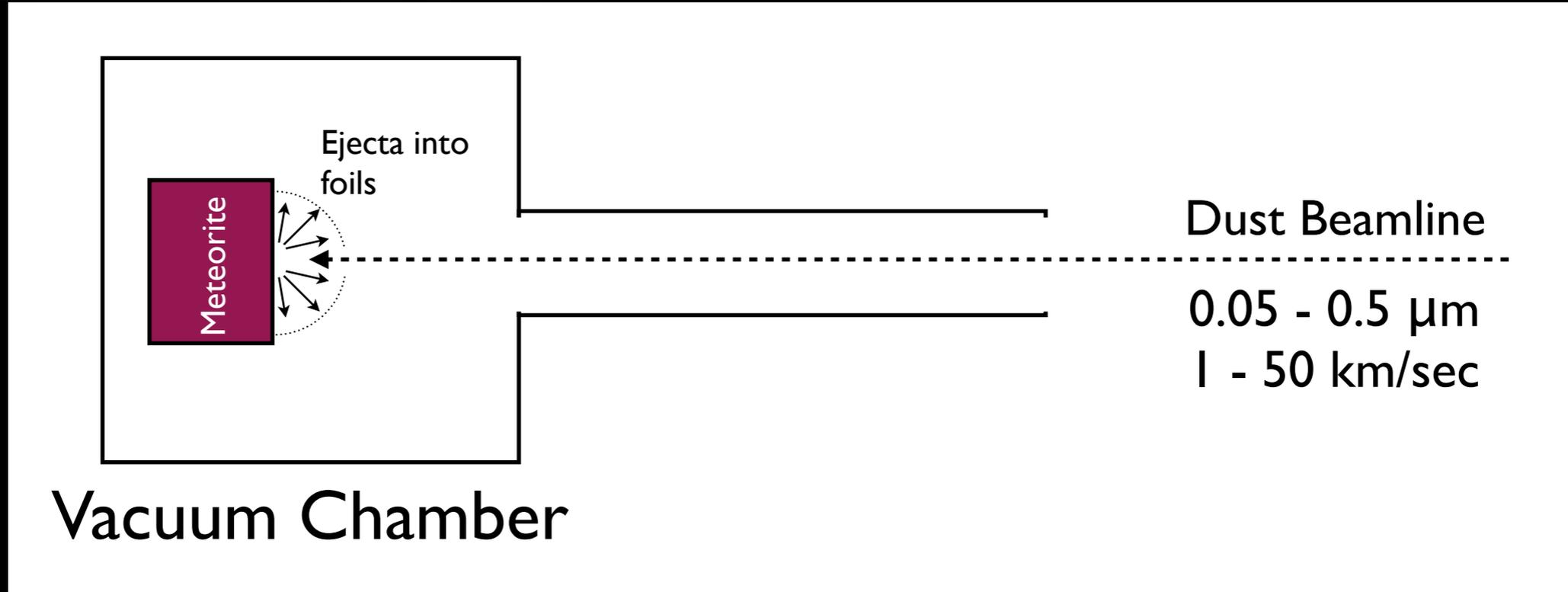
For science runs, we place foils to intercept ejecta in chamber to measure ejecta size.
