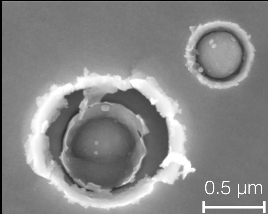
Two Fe grains embedded into Cu mesh.
