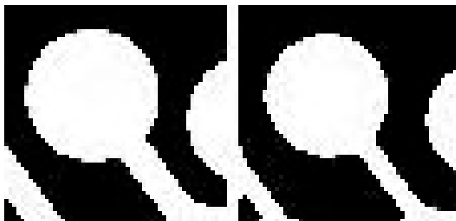
Figure 106. Original Image (left) and Eroded Image (right)
