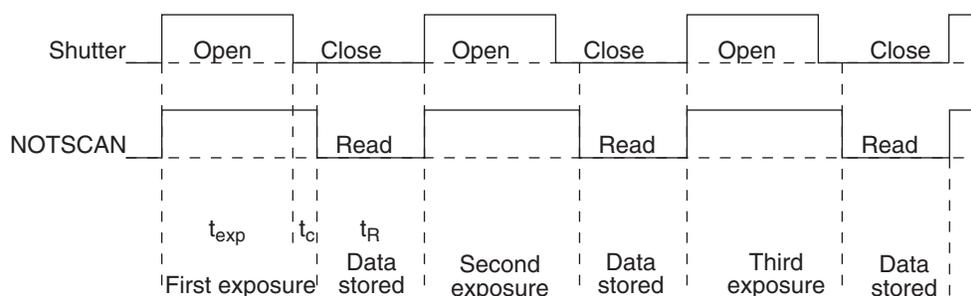
Figure 17. Free Run Timing Diagram
