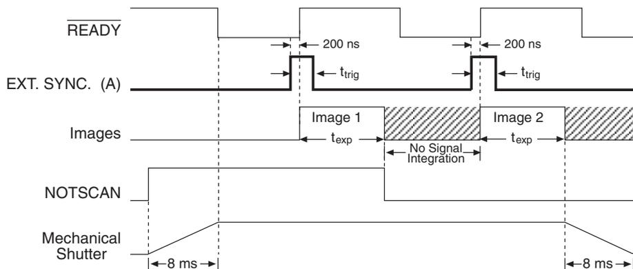
Figure 44. ESABI Timing Example: Image Exposure time =  $t_{exp}$  set in software
