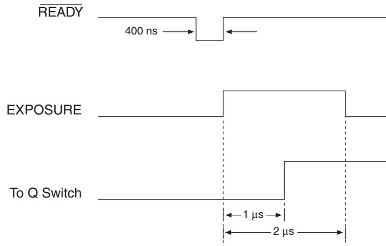
Figure 38. Timing for Experiment Setup shown in Figure 37
