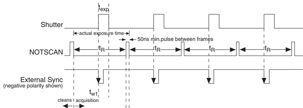
Figure 22. Frame Transfer where  $t_{w1} + t_{exp} + t_c < t_R$
