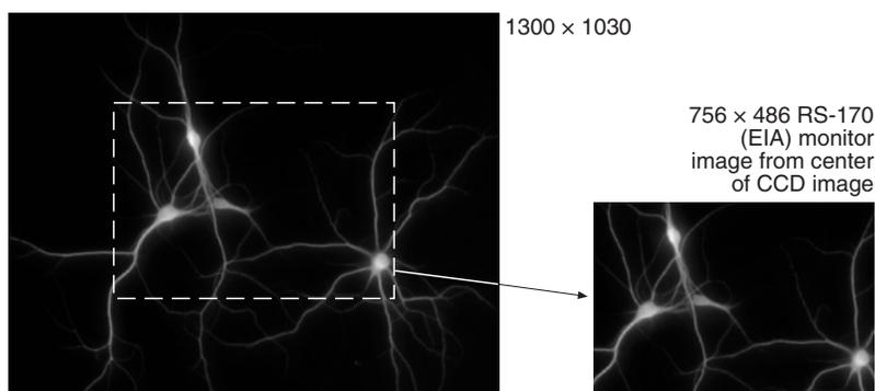
Figure 12. Monitor Display of CCD Image Center Area
