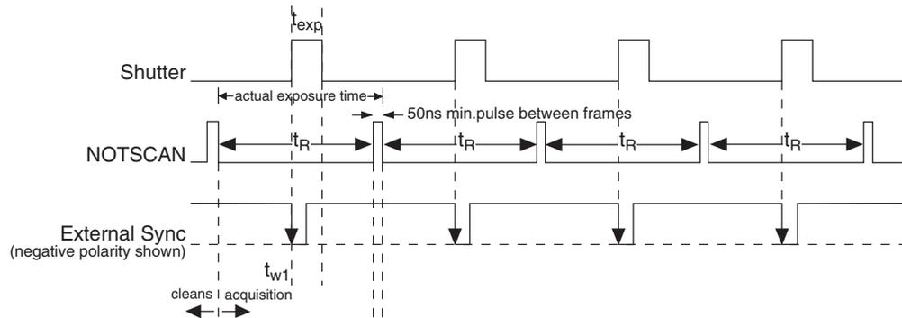
Figure 25. Overlapped Mode where  $t_{w1} + t_{exp} + t_c < t_R$
