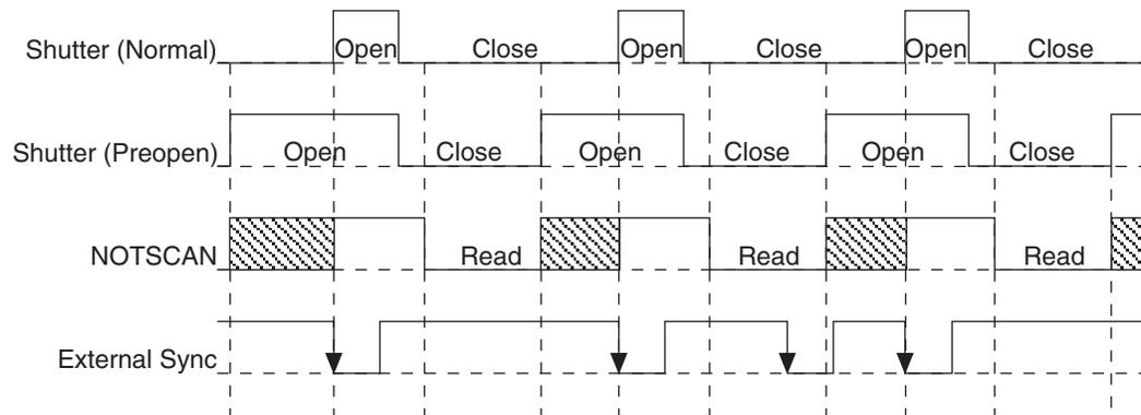
Figure 21. Continuous Cleans Timing Diagram
