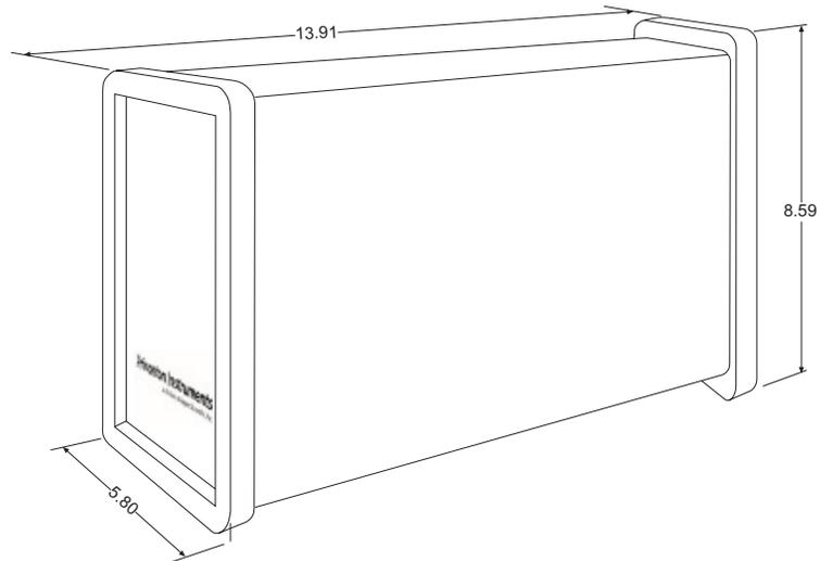
Figure 67. ST-133B Controller Dimensions
