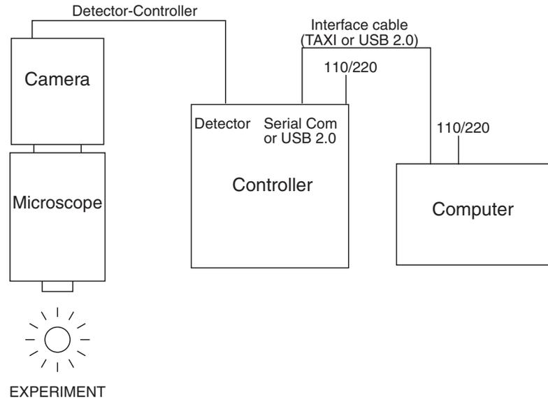
Figure 13. Standard System Connection Diagram
