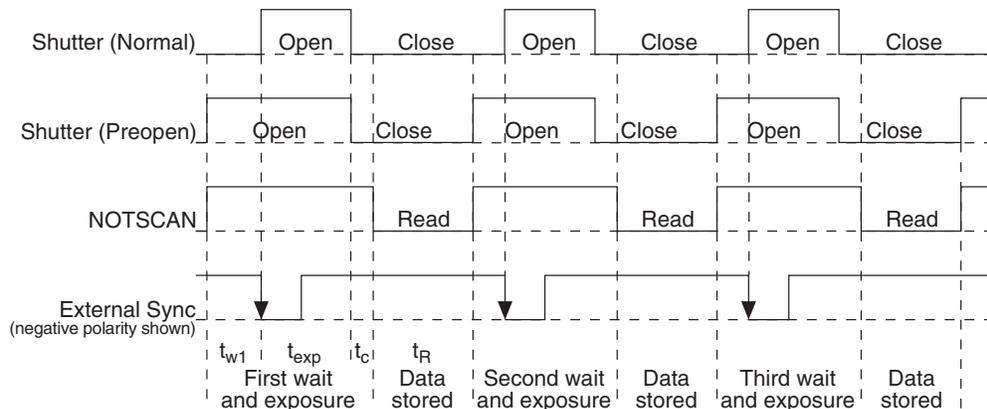
Figure 19. External Sync Timing Diagram (- edge trigger)
