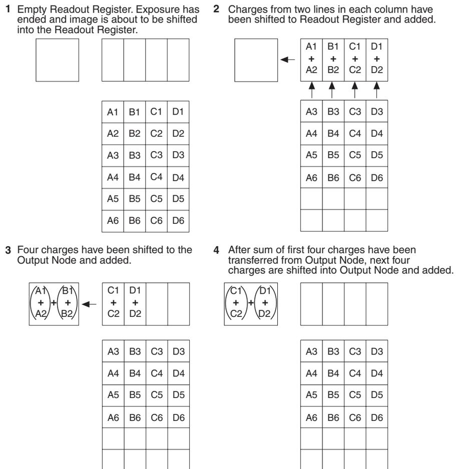
Figure 34.  $2 \times 2$  Binning for Full Frame CCD
