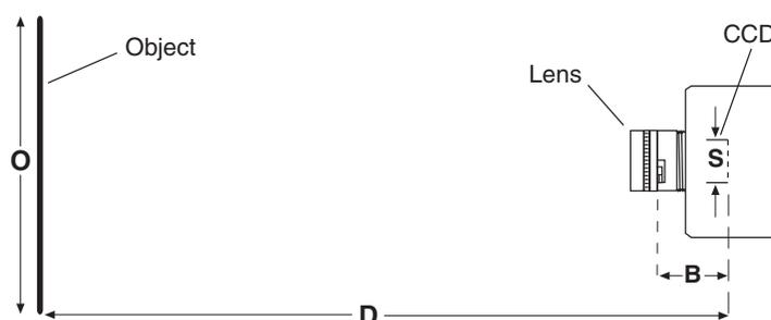
Figure 11. Imaging Field of View
