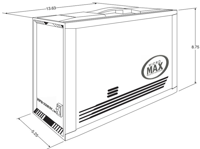
Figure 68. ST-133A Controller Dimensions
