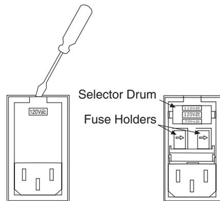
Figure 49. Power Input Module
