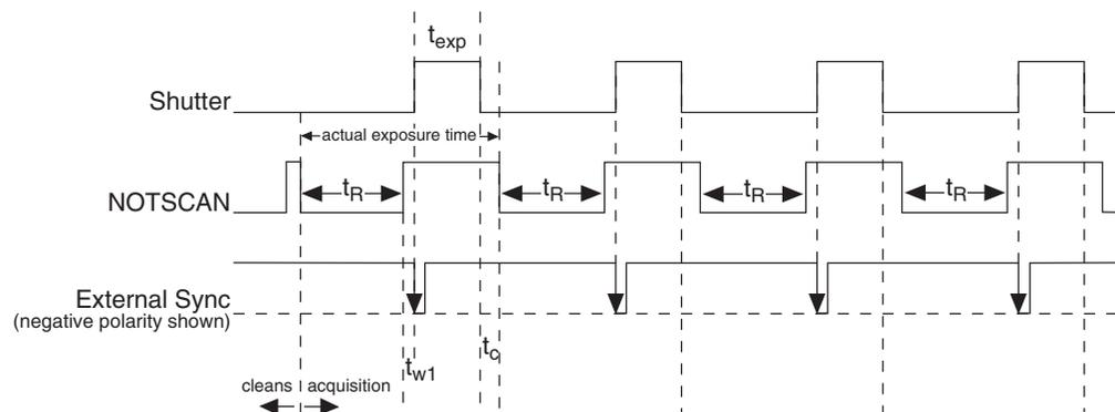
Figure 27. Overlapped Mode where Pulse arrives after Readout
