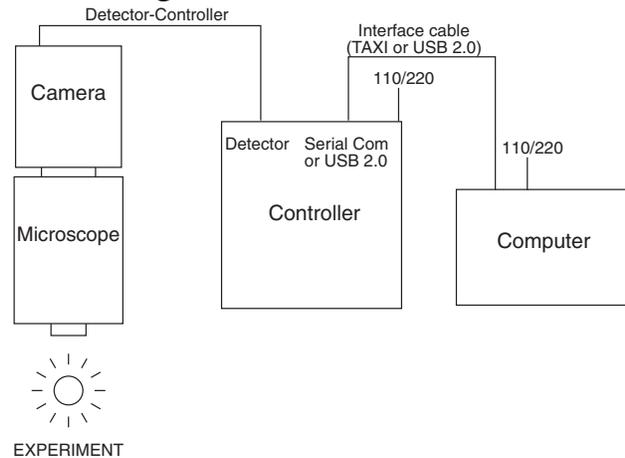
Figure 76. System Diagram
