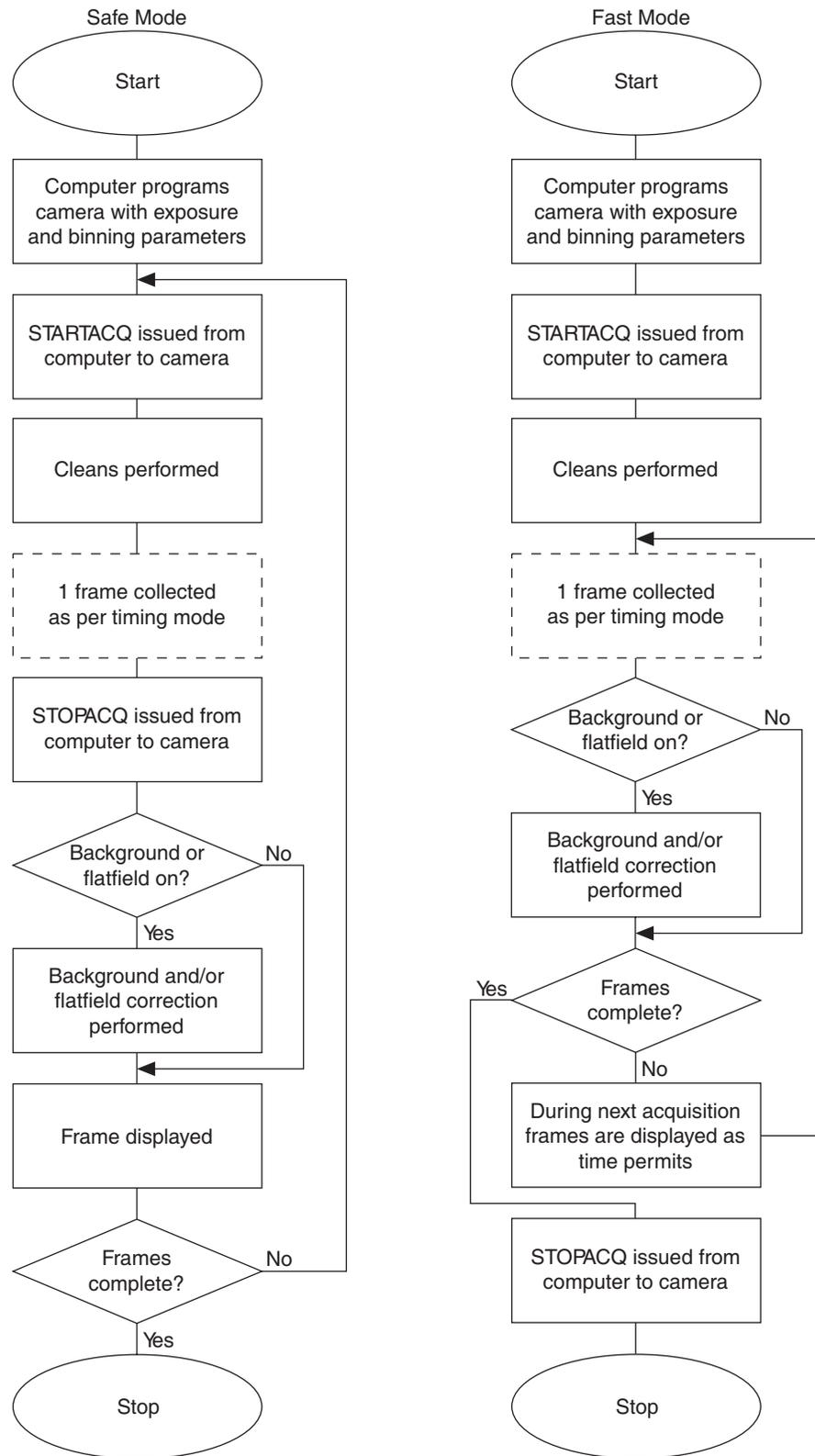
Figure 15. Chart of Safe and Fast Mode Operation
