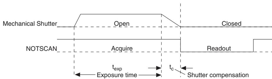
Figure 29. CCD Exposure with Shutter Compensation
