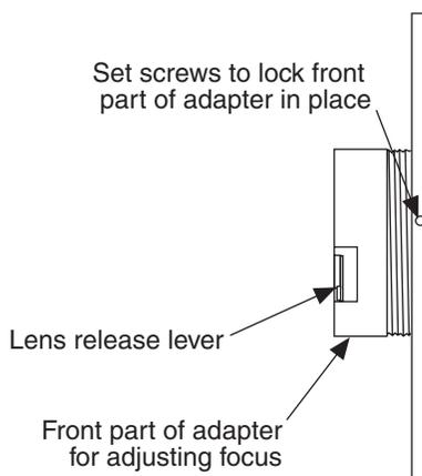
Figure 14. F-mount Focus Adjustment
