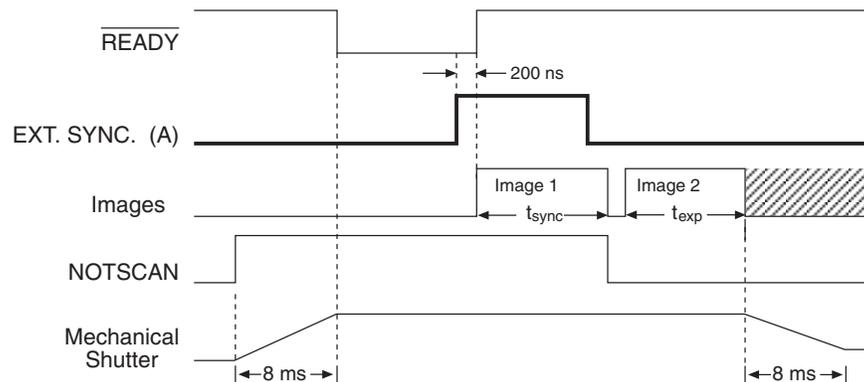
Figure 43. EEC Timing Example with Exposure Time in Software Set to  $t_{exp}$
