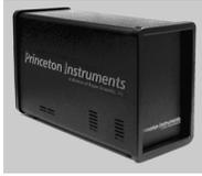
**Electronics:** The Model ST-133 is a compact, high performance CCD Camera Controller for operation with Princeton Instruments cameras. Designed for high speed and high performance image acquisition, the ST-133 offers data transfer at speeds up to 5 megapixel per second, standard video output for focusing and alignment. A variety of A/D converters are available to meet different speed and resolution requirements.
