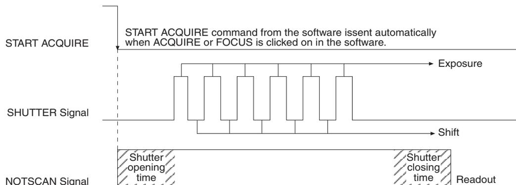
Figure 72. Free Run Timing Diagram
