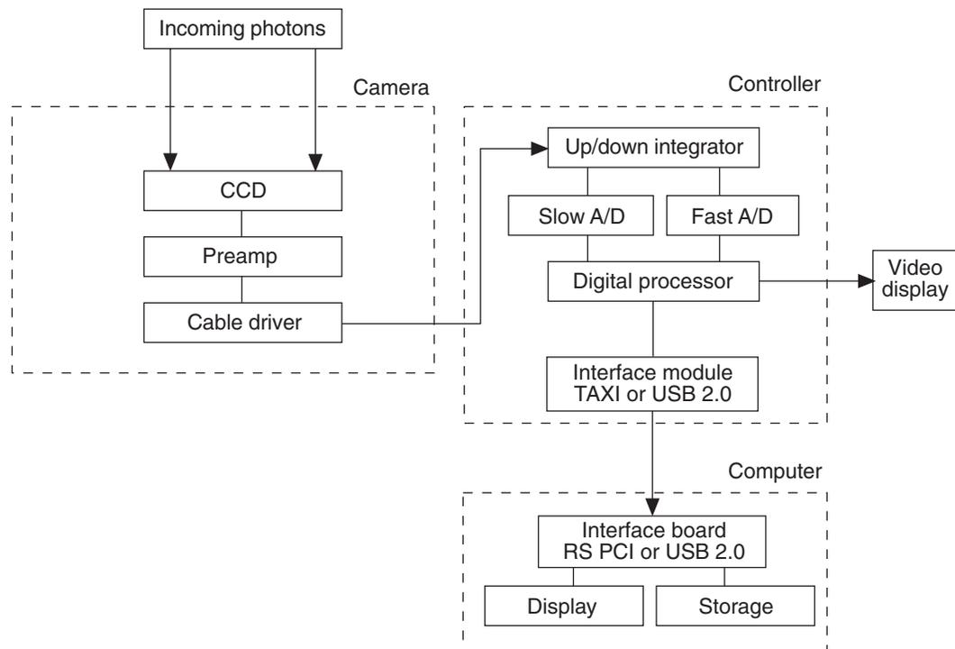
Figure 28. Block Diagram of Light Path in System
