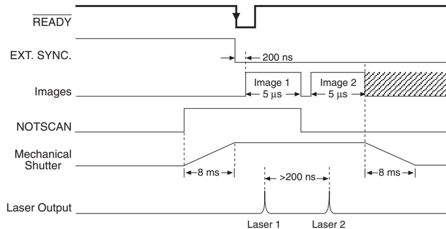
Figure 41. Timing Diagram for IEC Experiment with Two Lasers
