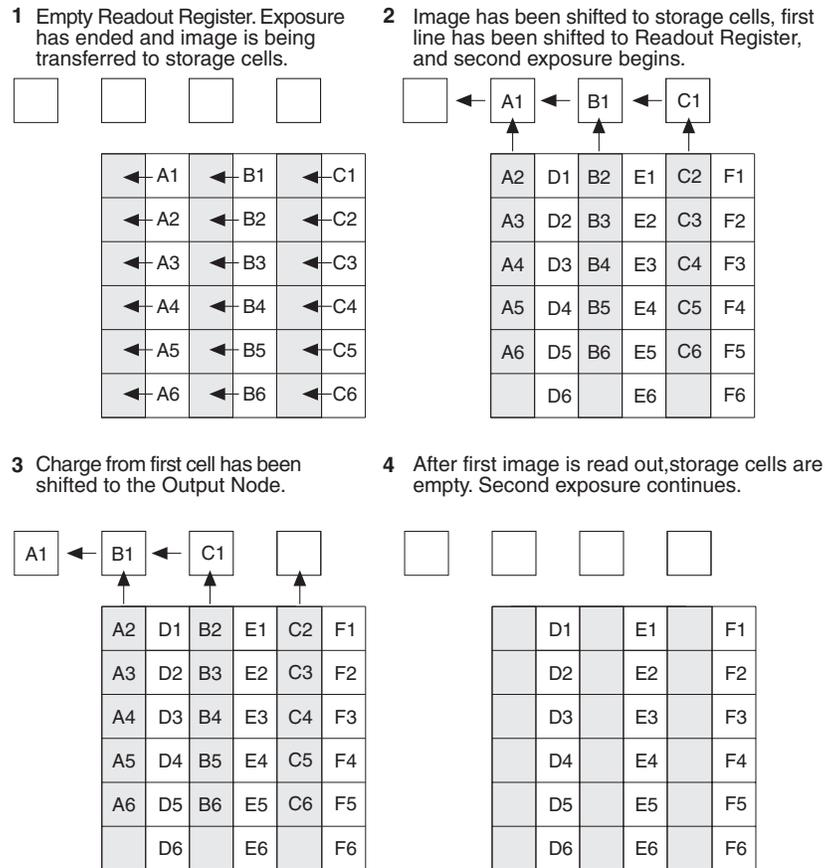
Figure 32. Overlapped Mode Exposure and Readout
