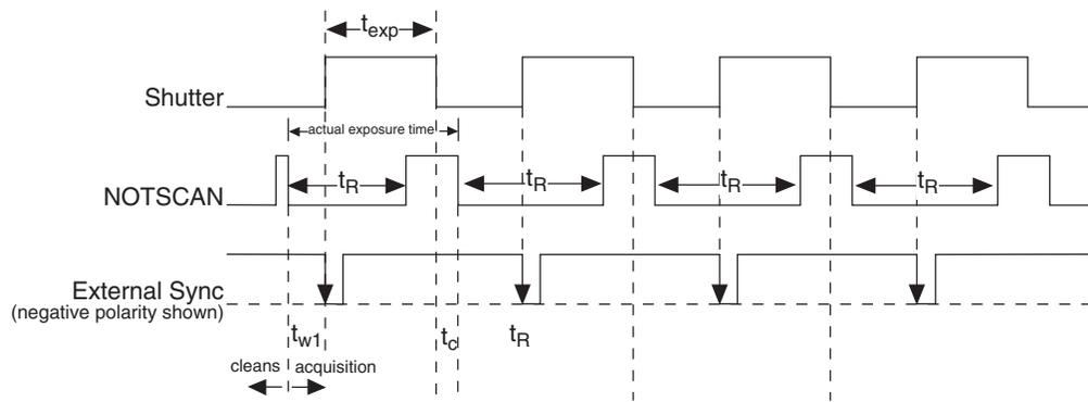
Figure 26. Overlapped Mode where  $t_{w1} + t_{exp} + t_c > t_R$
