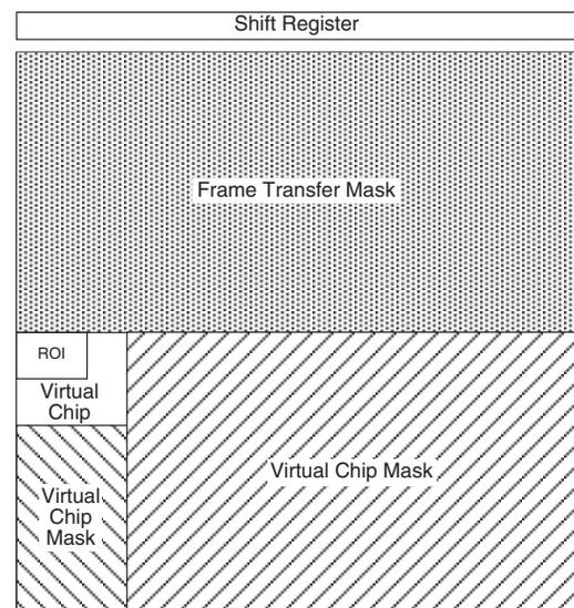
Figure 75. Virtual Chip Functional Diagram
