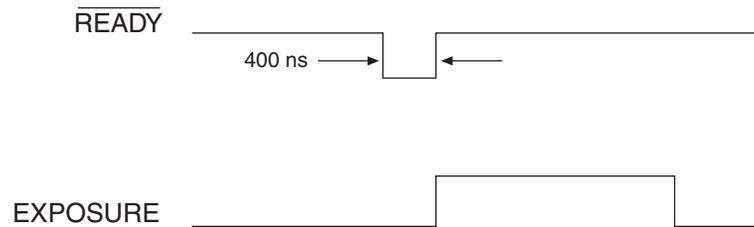
Figure 36. Free Run Mode Timing Diagram
