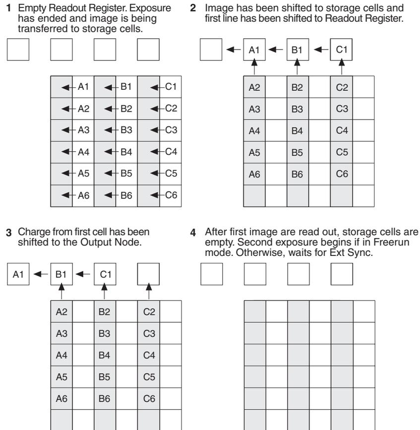
Figure 33. Non-Overlapped Mode Exposure and Readout
