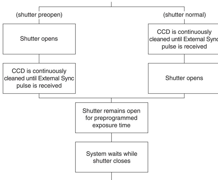
Figure 20. Continuous Cleans Flowchart
