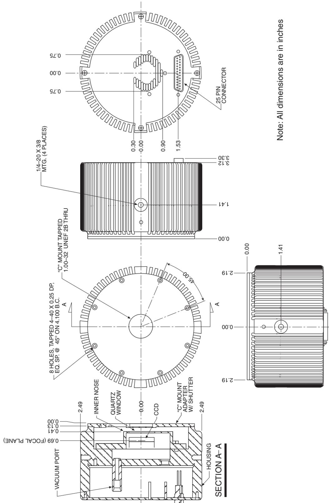
Figure 65. 1 MHz and 100kHz/1MHz Round Head Camera: C-Mount Adapter and Shutter
