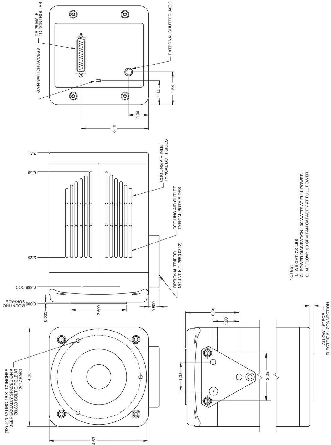
Figure 63. Rectangular Camera Head: Spectroscopy Mount with Shutter
