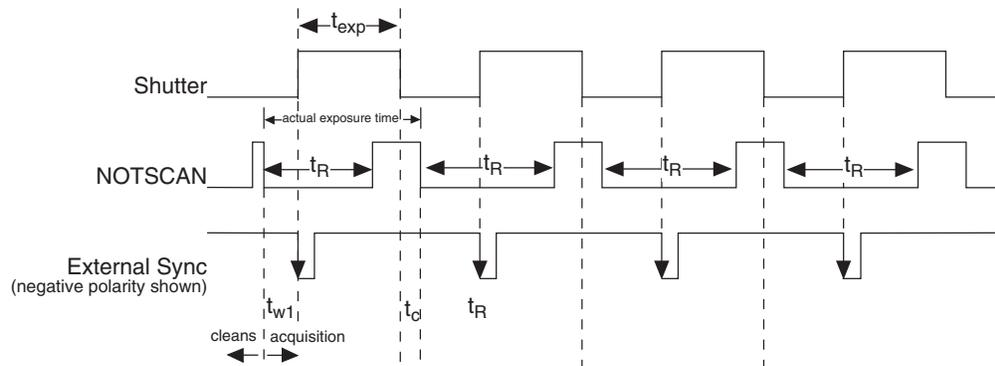
Figure 23. Frame Transfer where  $t_{w1} + t_{exp} + t_c > t_R$
