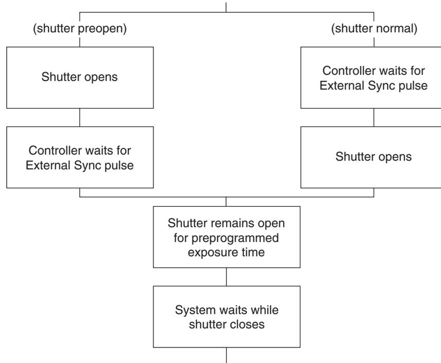
Figure 18. Showing Shutter "Preopen" & "Normal" Modes in External Sync Operation
