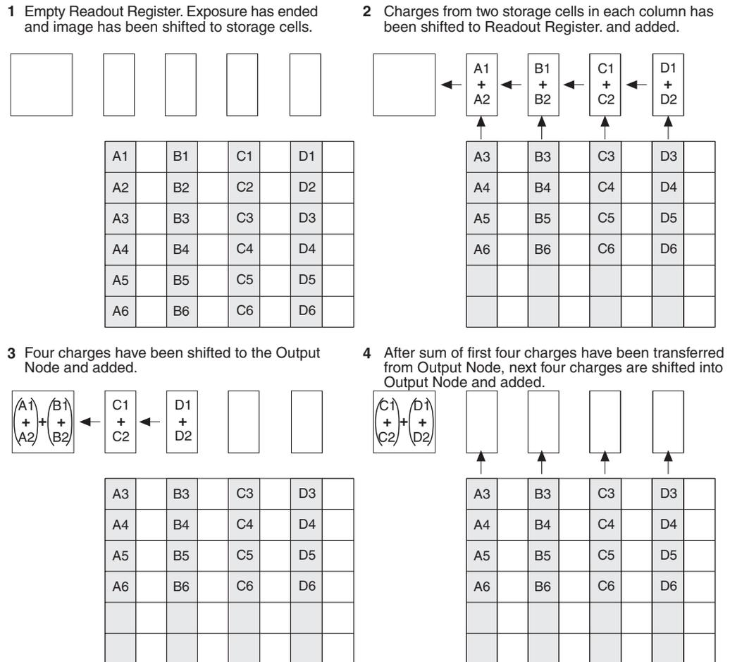
Figure 35.  $2 \times 2$  Binning for Interline CCD
