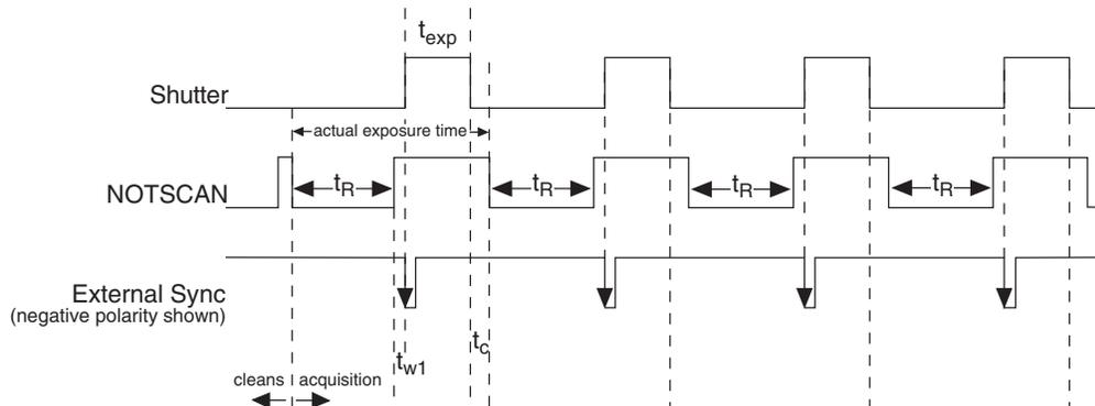
Figure 24. Frame Transfer where Pulse arrives after Readout
