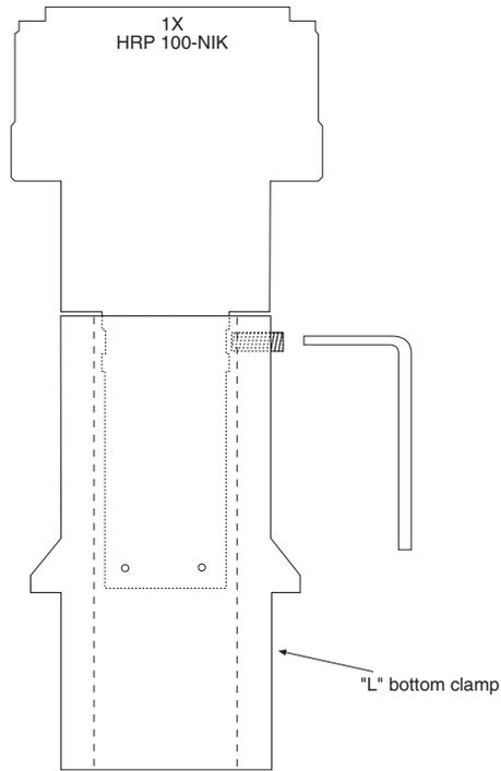
Figure 8. Bottom Clamp secured to Relay Lens
