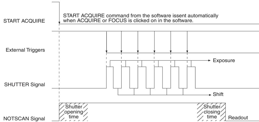
Figure 74. Multiple Trigger Timing Diagram
