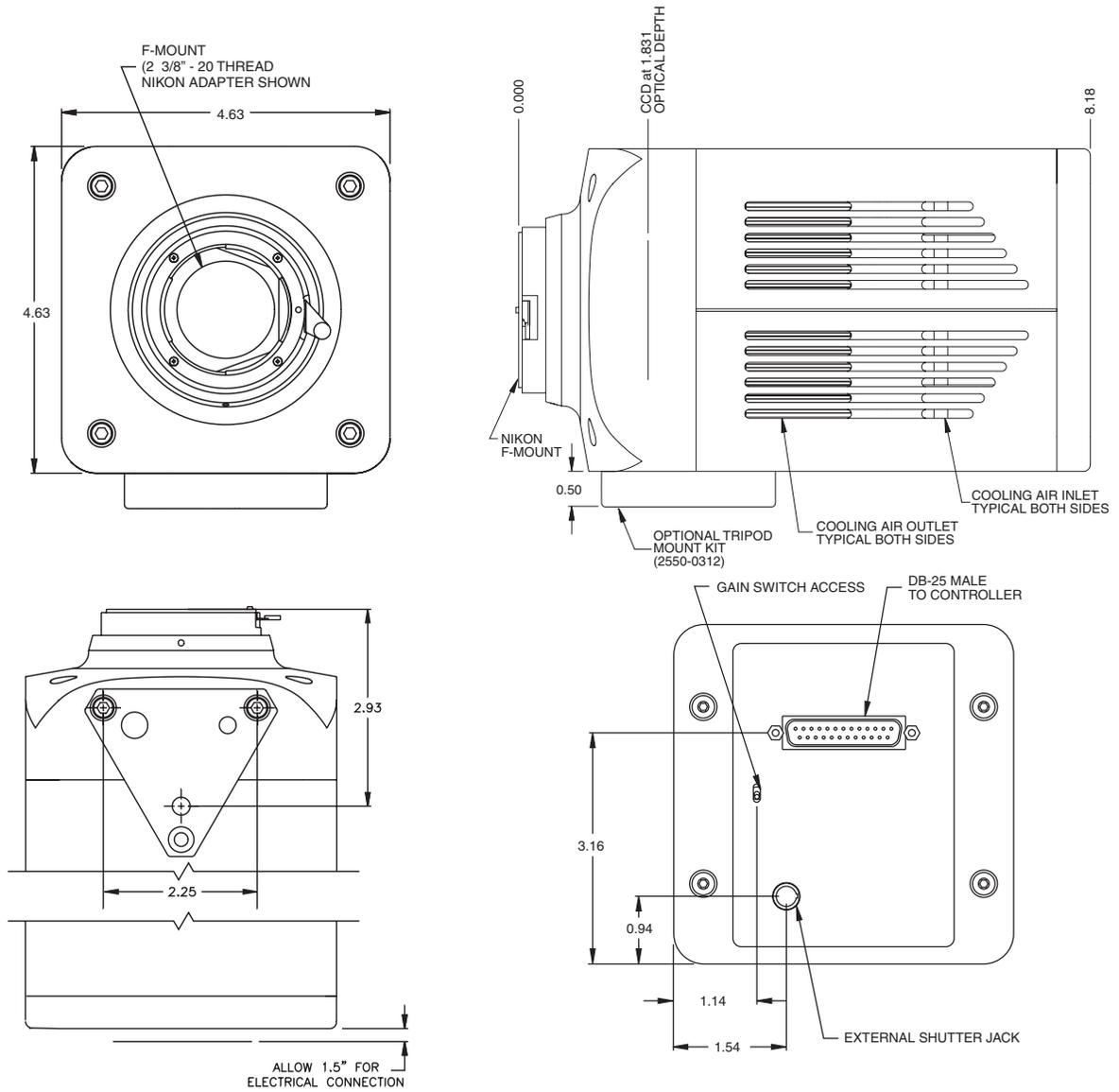
Figure 62. Rectangular Camera Head: F-Mount
