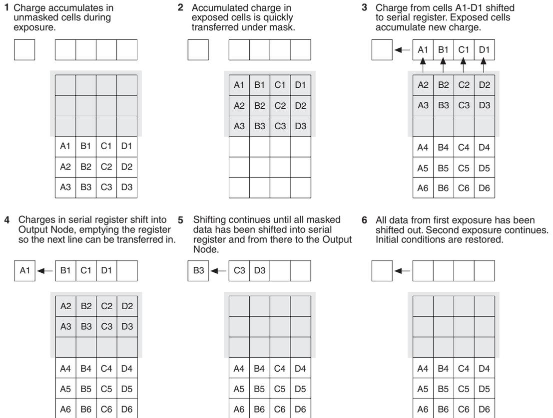
Figure 31. Frame Transfer Readout
