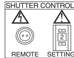
Figure 9. Shutter Setting for 25mm Internal Shutter
