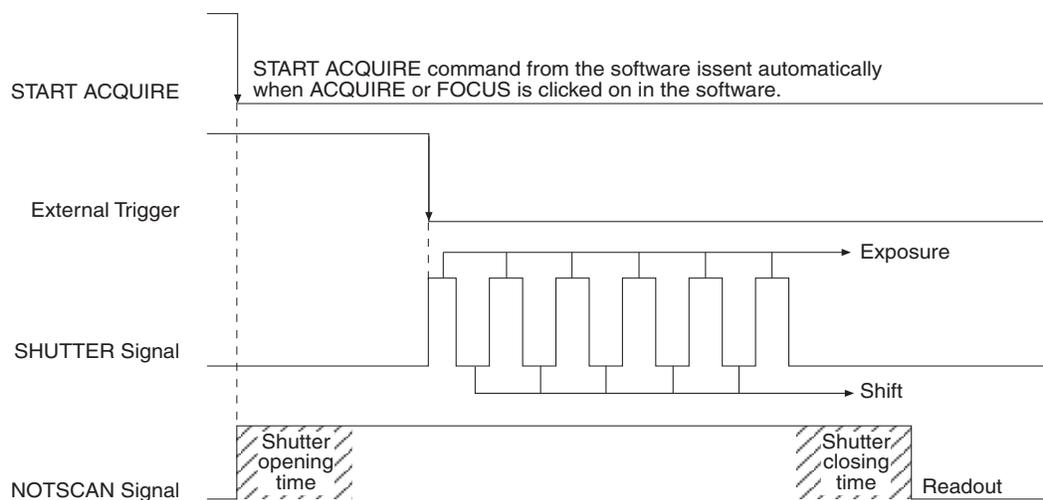
Figure 73. Single Trigger Timing Diagram
