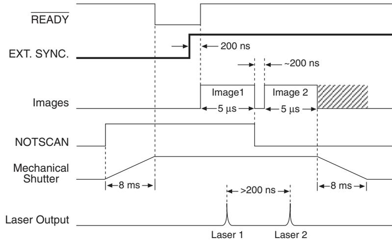
Figure 39. Timing Diagram for Typical IEC Measurement
