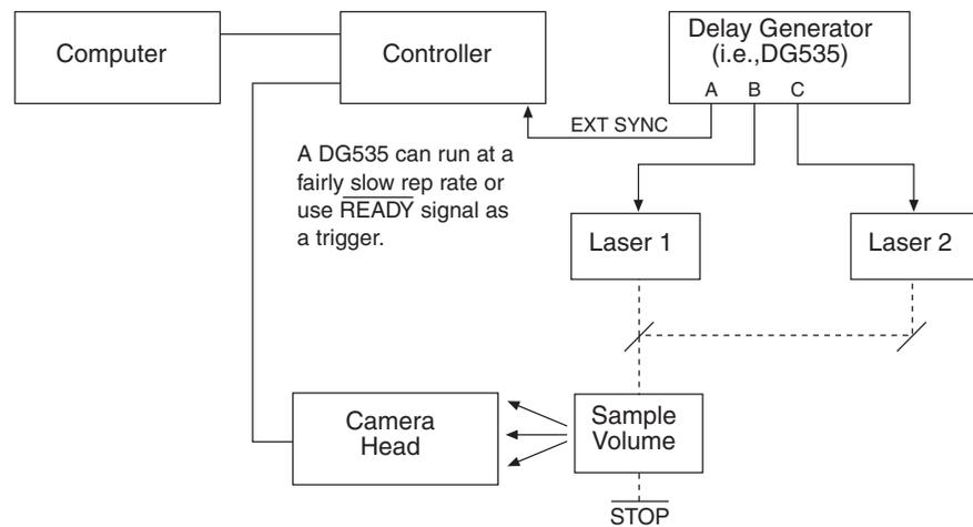
Figure 40. Setup for IEC Experiment with Two Lasers
