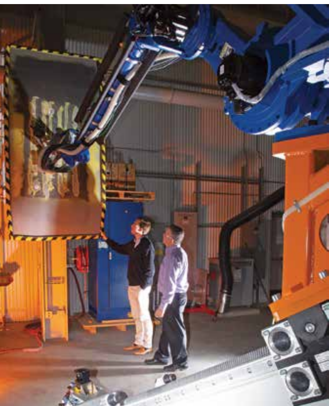
For nearly 50 years, SwRI has developed large-scale robot systems to perform aircraft maintenance. This system, designed to robotically "depaint" the F-22 stealth aircraft, was the largest fully robotic system of its kind when it was installed at Hill AFB in 2011.
