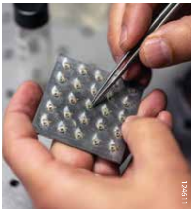
The SwRI method allows batch testing. Microspheres loaded into this miniature series of “barrel” holes allow the system to automatically fire them in rapid succession.
