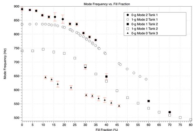
**Figure 3:** Variation of representative mode frequencies with fill fraction for both 1-g settled fluid configurations and 0-g slosh-averaged fluid. Error bars on the flight data represent standard error in the data, while error bars for the 1-g data are not depicted, but would be smaller than the data symbol.
