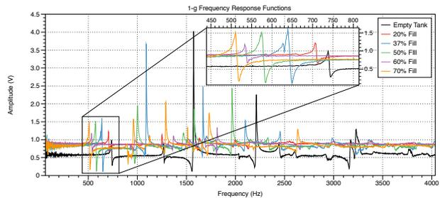
**Figure 1:** 1-g Frequency Response Functions recorded for settled fluid with tank in vertical position. Inset shows blow-up of fundamental mode and demonstrates the decrease of mode frequency with increasing fill-fraction.
