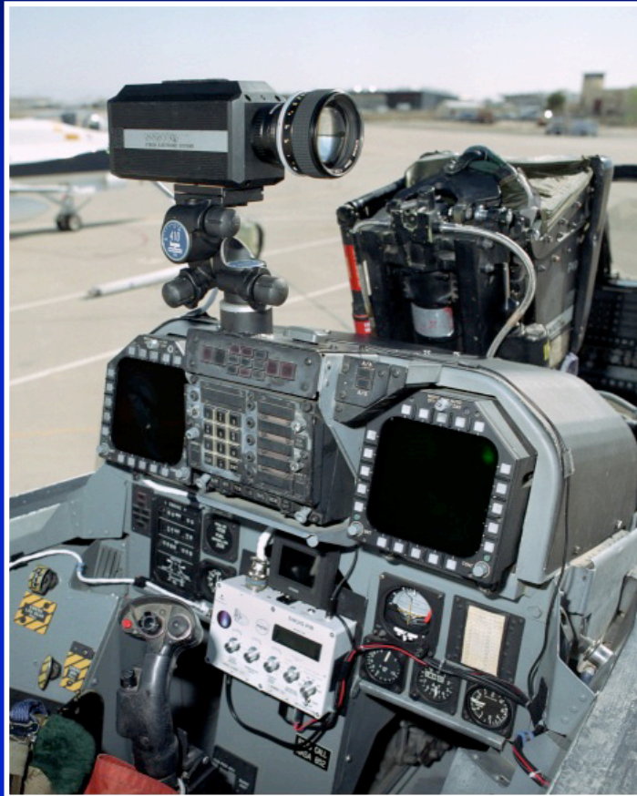
SWUIS-A installed in F-18 aft cockpit
