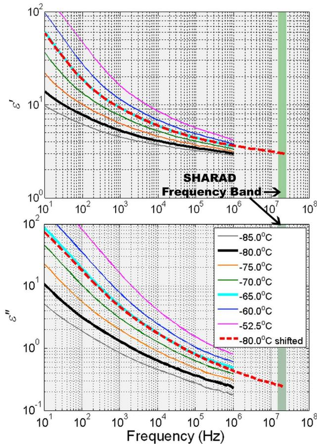
**Figure 6.** Our laboratory measurements of the low-frequency dispersion due to three monolayers of 1 M  $\text{CaCl}_2$  aqueous solution on sand mixed with 9.67 vol % STx-1. Because the relaxation frequency follows a simple Arrhenius activation energy, we can extrapolate (top)  $\epsilon'$  and (bottom)  $\epsilon''$  to SHARAD frequency simply by laterally shifting cold temperature data ( $-80^\circ\text{C}$ ) to the desired temperature ( $-65^\circ\text{C}$ ).
