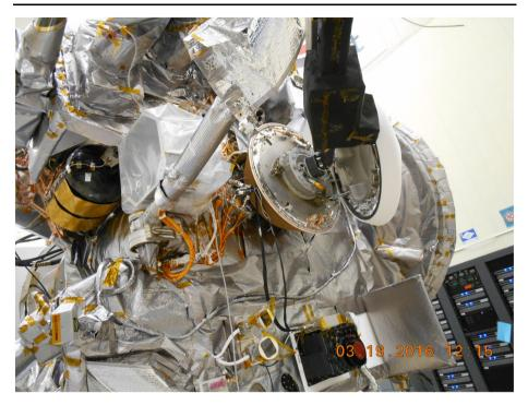
Fig. 36 The spacecraft's TAGSAM head is placed into the Sample Return Capsule during a stowage verification test executed at Lockheed Martin's cleanroom (Lockheed Martin)
