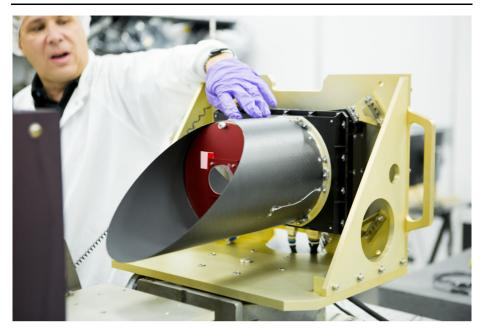
**Fig. 17** The OSIRIS-REx Thermal Emissions Spectrometer, provided by Arizona State University, determines mineral and temperature information by collecting infrared (from 5 to 50 microns) spectral data from Bennu (Arizona State University)
