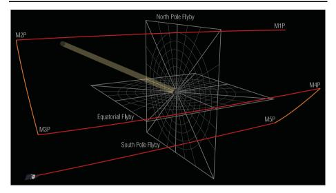
**Fig. 27** The OSIRIS-REx spacecraft's Preliminary Survey orbit path. The spacecraft will complete five legs to allow for flybys of Bennu's North Pole, Equator and South Pole, using trajectory changes at the Maneuver 1 Preliminary Survey (M1P) though Maneuver 5 Preliminary Survey (M5P) points
