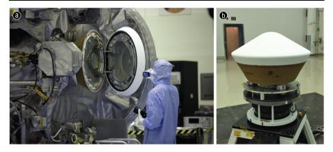
**Fig. 13** The Sample Return Capsule is the only part of the OSIRIS-REx spacecraft that will return to Earth at the end of the mission. (a) A technician inspects the open capsule during testing. (b) The closed SRC sits in a Lockheed Martin cleanroom (Lockheed Martin)
