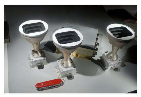
Fig. 19 The TAGCAMS flight unit built by Malin Space Science Systems. The two Navcams are at the left and center and the Stowcam is on the right. The digital video recorder is behind the center camera head, containing two separate recorder boards. The pocketknife is for scale (Malin Space Science Systems)
