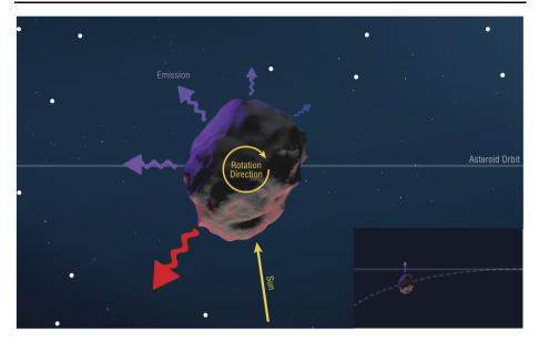
**Fig. 4** The Yarkovsky effect causes the orbit of a small body to change over time. As the heat absorbed from the sun during the day is emitted from the night side of the asteroid, a small but continuous thrust is created which pushes the asteroid out of its normal orbit
