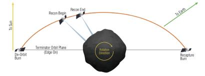
Fig. 32 Diagram of the spacecraft's Reconnaissance Phase trajectories that will provide greater detail on the selected primary and secondary sampling sites
