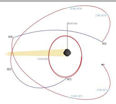
**Fig. 29** Trajectory diagram for the "Baseball Diamond" maneuver, which begins the mission's Detailed Survey Phase. The spacecraft will progress through a series of hyperbolic passes around Bennu, with trajectory changes at the Maneuver 1 Detailed Survey (M1D) through Maneuver 5 Detailed Survey (M5D) points
