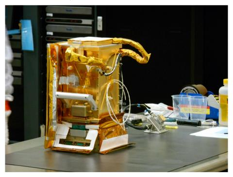
Fig. 18 The Regolith X-ray Imaging Spectrometer (REXIS), a student-built instrument, will determine which elements are present on the surface of Bennu (MIT)
