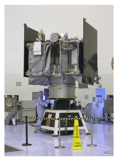
Fig. 8 The OSIRIS-REx spacecraft installed on a rotation fixture in a NASA Kennedy Space Center clean-room in preparation for launch (NASA)
