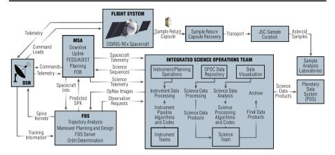
Fig. 21 Diagram outlining the OSIRIS-REx ground system, its products and its dependencies
