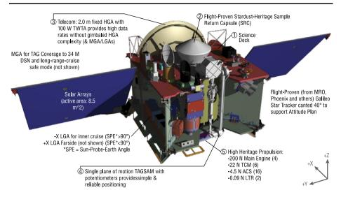
Fig. 9 CAD drawing of the OSIRIS-REx spacecraft depicting its principal components
