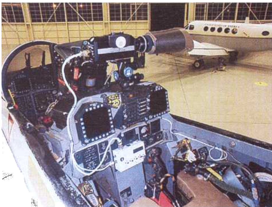
Fig. 1. (Top panel) NASA F/A-18B aircraft used for flight testing the SWUIS-A instrument system at the Dryden Flight Research Center in Edwards, California, USA. The SWUIS-A flight astronomer operates the instrument from the rear cockpit. (Bottom panel) The SWUIS-A system integrated into a NASA F/A-18B. The aircraft-to-camera power and telemetry interface (PIB) and LCD monitor are visible just in front of the stick. White cables running from the PIB to the right side of the cockpit connect to the aircraft power supply and video tape recorder. The Xybion ICCD camera is mounted above the instrument panel glare shield. On this flight, the 85 mm f/1.4 foreoptic was mounted on the camera, here with a foam light baffle attached.
