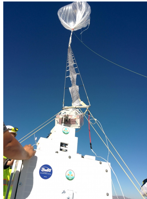
B-SSIPP launched under a World View envelope on 1-Nov-2019, achieving 97,000 ft altitude and observing the Sun in the spectroscopic “g-band”.
