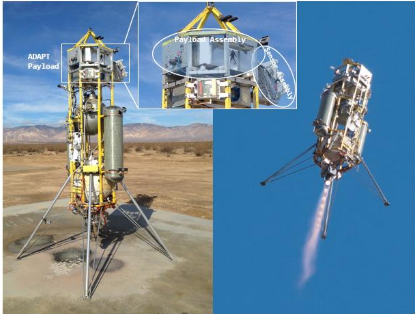
Figure 2. ADAPT installed on the Xombie VTVL rocket vehicle, on the ground (left) and in flight (right, image credit NASA Photo / Tom Tschida).
