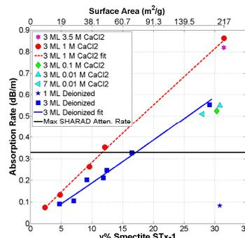
**Figure 2.** Absorption rate of SHARAD energy at  $-65^\circ\text{C}$  with 1-7 monolayers (ML) with differing amounts of  $\text{CaCl}_2$ .  $\text{CaCl}_2$  concentrations of  $> 1\text{M}$  with 3 ML lead to a 50% jump in the absorption rate. As the number of monolayers is increased to three,
